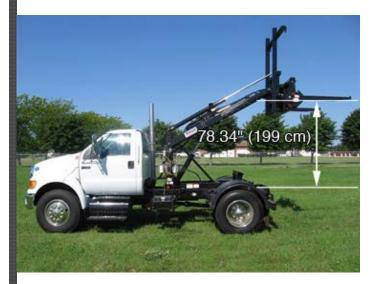
From the top of the frame rail to the bottom of the fork is 78.34" (199 cm).
